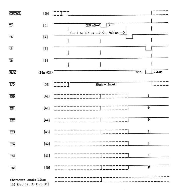
Figure 450-2: Timing Diagram for ASCII Character 9 Input
