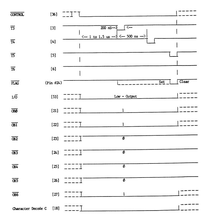
Figure 450-1: Timing Diagram - Output Character C from System Controller
